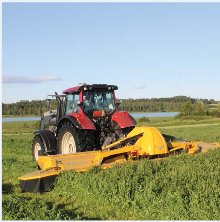
In reverse driving the object is directly in front of the driver, which promotes the ease of work. Photos: Markku Lätti
