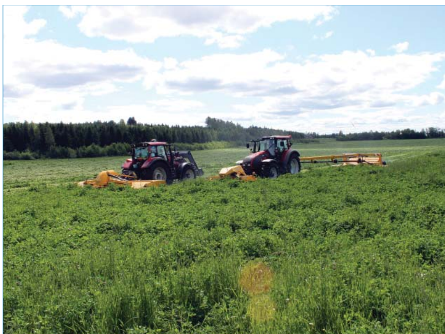
In both tractor-machinery combinations, the vibration measured from the driver's seat was clearly under the action value of 0.5m/s^2 for body vibration.
