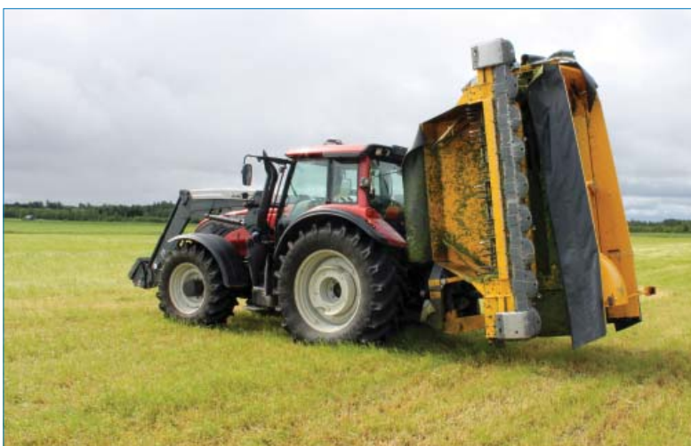
The sideflows of the mower conditioner can be lifted up with a push of a button during transportation.
