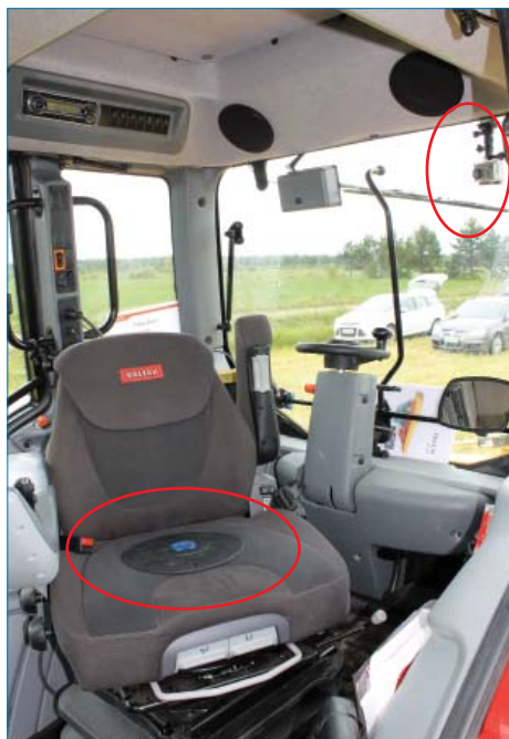
Left: For the working posture study, the working postures of the driver were photographed with a miniature camera and body vibration was measured with a vibration sensor installed on the seat. Right: The seat during reverse drive.
