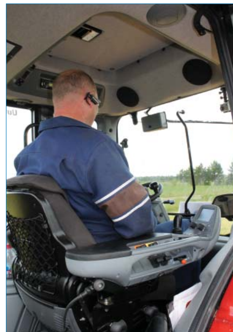
Left: For the working posture study, the working postures of the driver were photographed with a miniature camera and body vibration was measured with a vibration sensor installed on the seat. Right: The seat during reverse drive.
